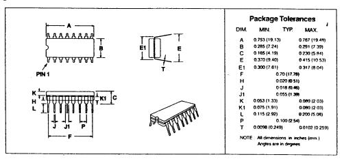
Figure 6: 16-pin CDIP Mechanical Outline: order as part no. MX316P
