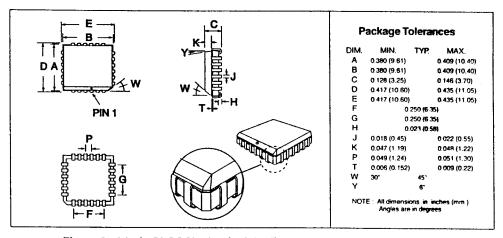
Figure 8: 24-pin PLCC Mechanical Outline: order as part no. MX316LH
